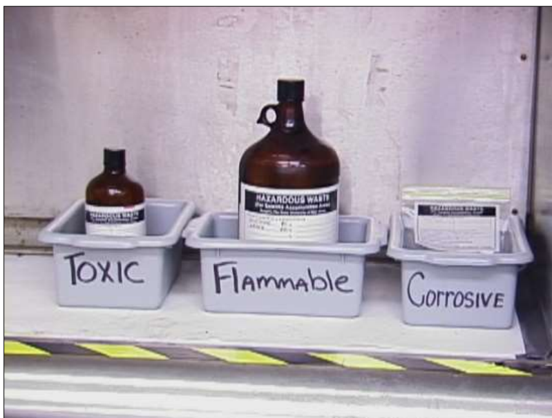
Figure 1. Example of Properly Stored Hazardous Waste in SAA
