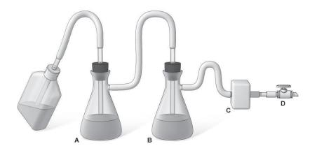
**Figure 2. Vacuum Line Protection: (A)** Collection Flask With Disinfectant; (B) Back-Up Flask (optional); (C) In-line HEPA filter; and (D) Connection to Building Vacuum.
