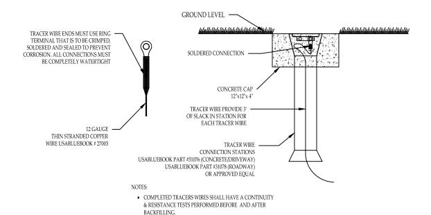
DURING BACKFILL CARE SHOULD BE TAKEN NOT TO DAMAGE TRACER WIRE INSULATION.
