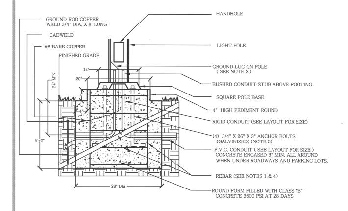
NOTES: SEE PLAN FOR LOCATIONS OF EXISTING FIXTURES TO REMAIN. PROVIDE GROUND ROD 3/4" X 8' AT EVERY OTHER POLE AND CONNECT TO GROUND LUGS IN POLE BASE & TO GROUND WIRE.
